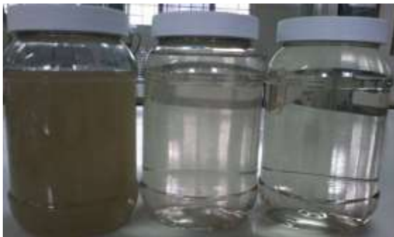
Figure 3. Visual comparison between the untreated wastewater (left), wastewater after treatment by biofilters (center), and wastewater after treatment by constructed wetland (right).
