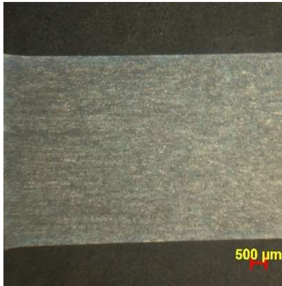
Figure 3. Macrograph of the base metal at 10X.
